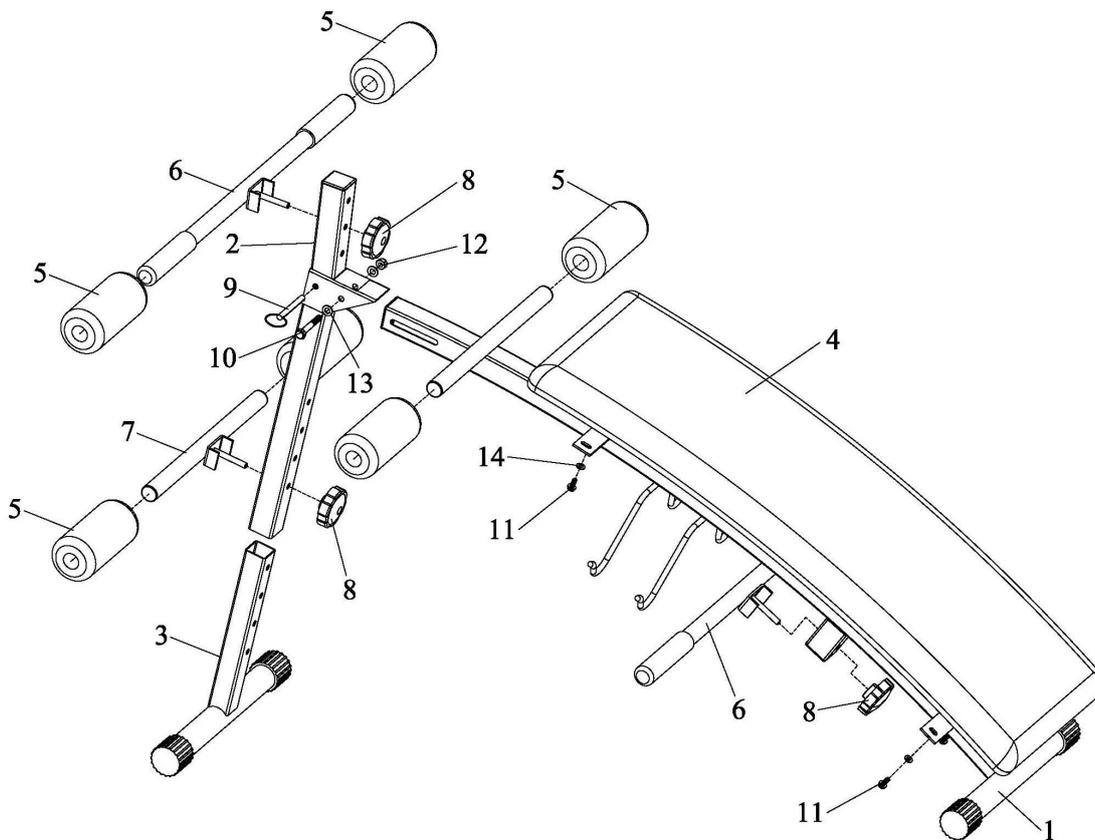
**STEP1** Fasten Back Rest (4) to Main Frame (1) with 4 Screws (11) and 4 washers (14).
